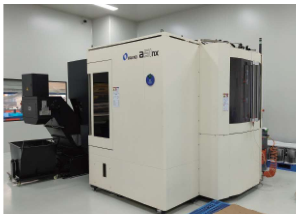
Japanese Makino horizontal 4-axis machining center
