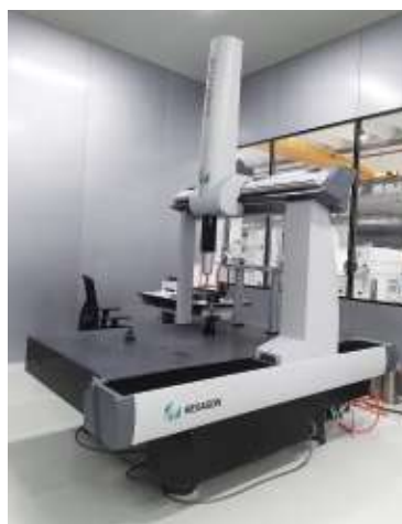
Coordinate measuring instrument Global plus 10.15.8 (including TP200 probe and HP-S-X1S probe)
