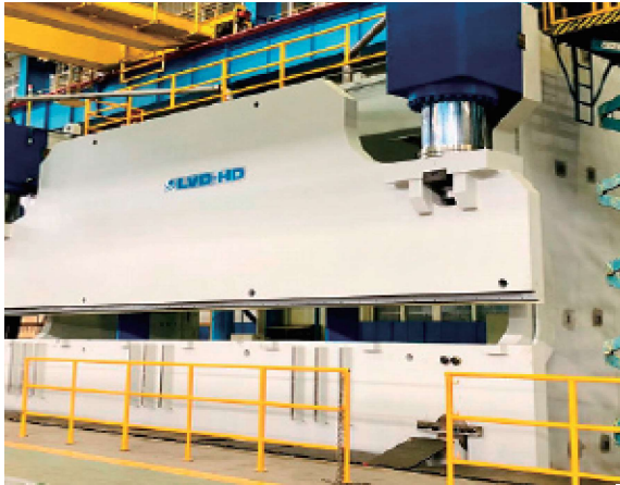
Belgian LVD-HD multi-axis electro-hydraulic servo CNC bending machine
