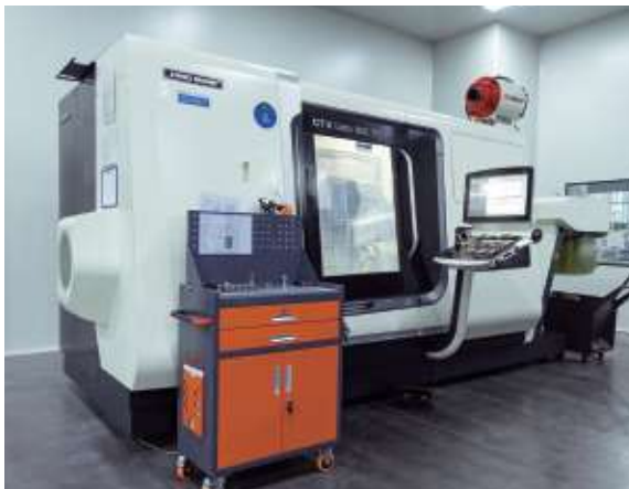
German original five-axis high-precision turning-milling compound machining center
