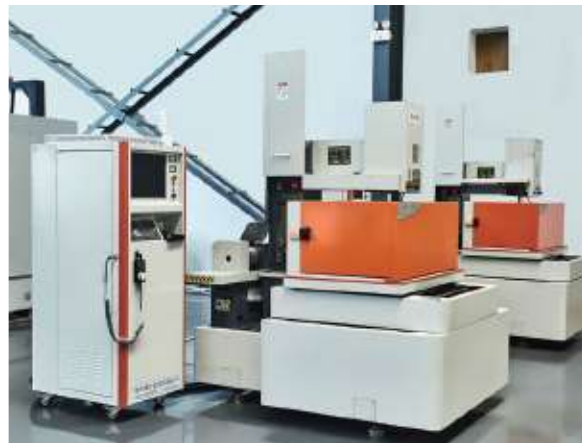
Medium-speed wire-cutting EDM machine
