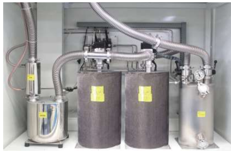
Purification system (molecular sieve and copper catalyst)
