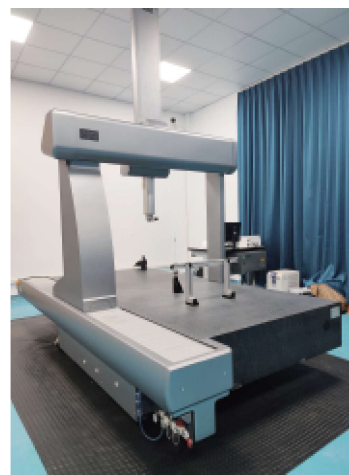
Coordinate measuring instrument GLOBAL S (including scanning probe)
